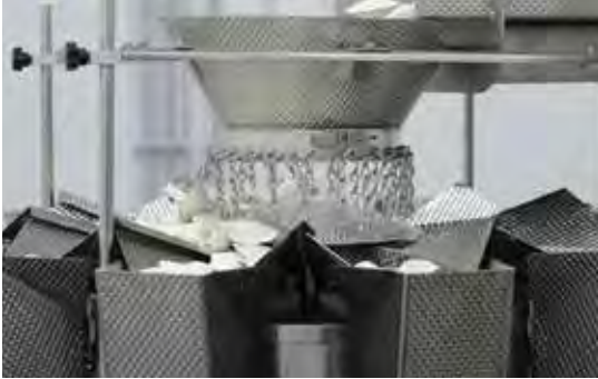
A high-speed feeder meters material into a packaging machine
